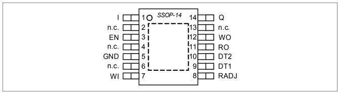
Figure 3 Pin Configuration
