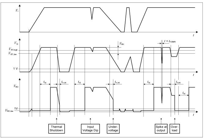
Figure 7 Typical Timing Diagram Reset
