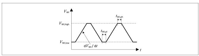
Figure 10 Test Pulses Watchdog Input WI
