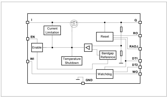
Figure 2 Block Diagram TLS820F1ELV50
