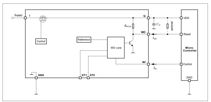
Figure 8 Block Diagram Watchdog Circuit
