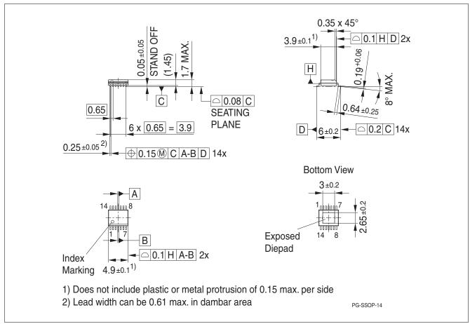
Figure 13 PG-SSOP-14
