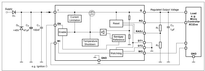
Figure 12 Application Diagram
